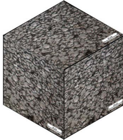
Figure 1 shows the microstructure of AZ31 in directions parallel and transverse to the rolling direction. (fine-grain structures are seen in the skin-layer.)
