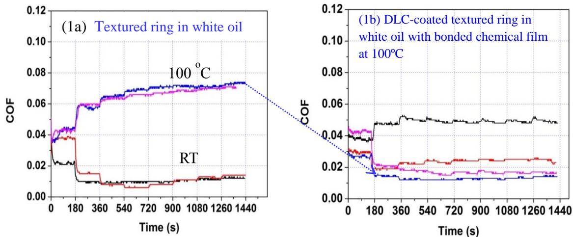
Fig. 1. The effect of temperature on the friction is shown in Fig. 1a; the effect of DLC and the bonded chemical film on top of DLC is shown in Fig. 1b.
