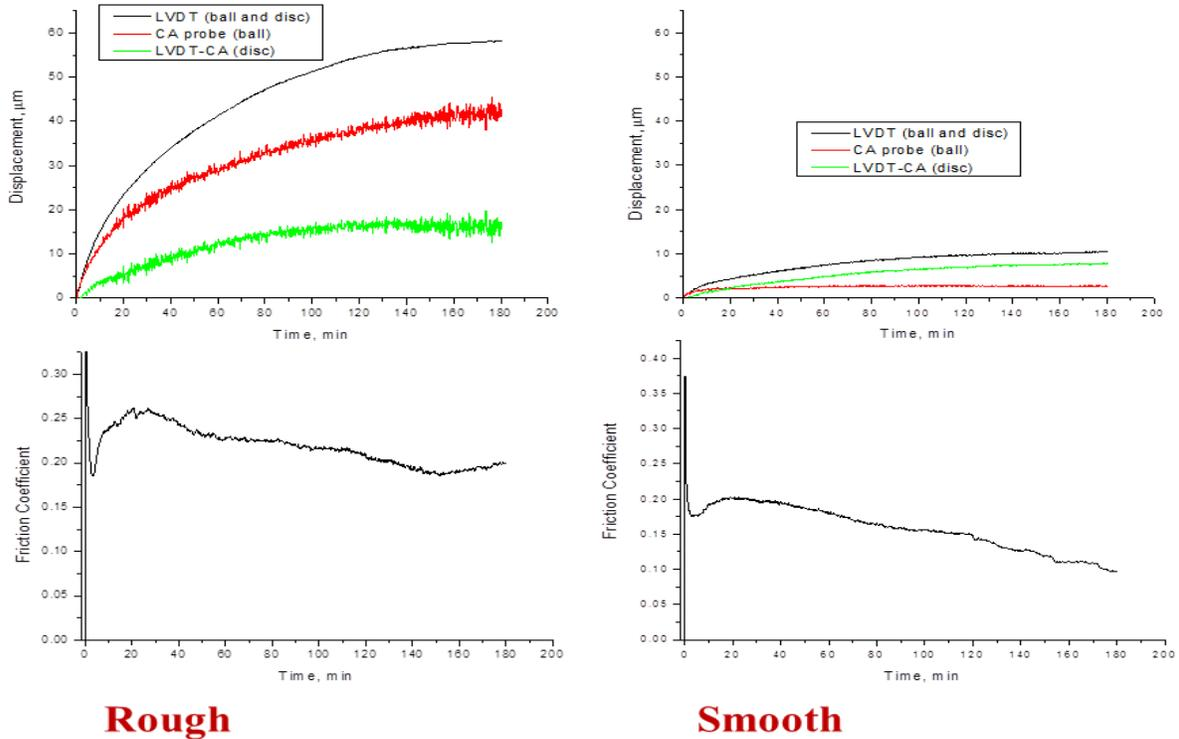
Fig. 4. Real-time pin-on-disk contact analysis of a rough and a smooth DLC coated surface carried out by National Physical Laboratory, UK.
