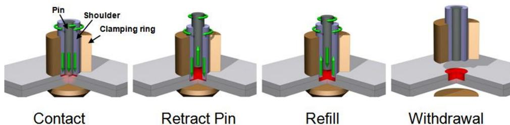
Fig. 5. Schematic diagram of the friction stir spot welding operation
