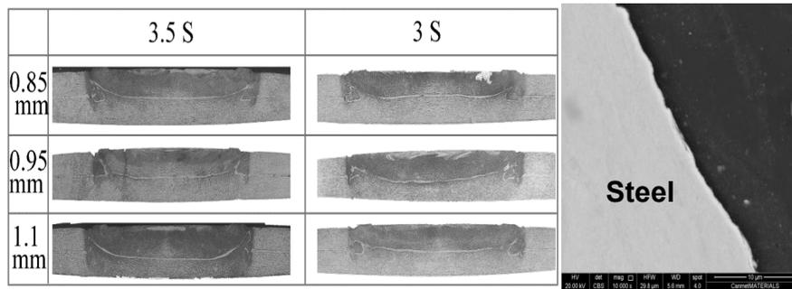
Fig. 6. Friction stir spot welding micrographs showing the weld interface
